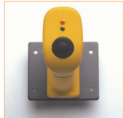
Position 3 (Red LED) STOP Function
