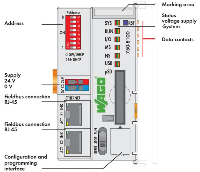
The PFC100 Controller is a compact PLC for the modular WAGO I/O-SYSTEM. In addition to providing commonly used network and fieldbus interfaces, the controller supports all digital, analog and specialty I/O modules in the 750/753 Series.
