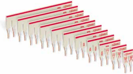
Staggered jumper (seven contacts) Individual jumper contacts can be broken off by bending them. The remaining piece of insulation will meet requirements for clearances and creepage distances.
