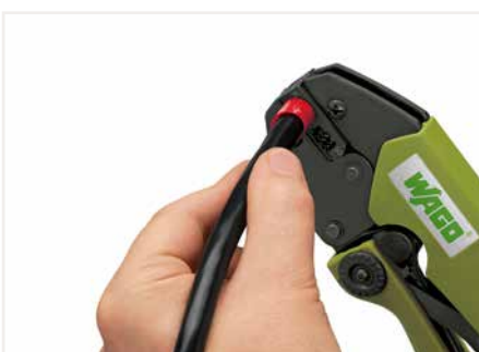
Squeeze handles until ratchet mechanism is released.
