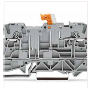
Variant: One disconnect and one through terminal block are accommodated on two levels in a terminal block that is just 5.2 mm (0.205 inch) wide.
