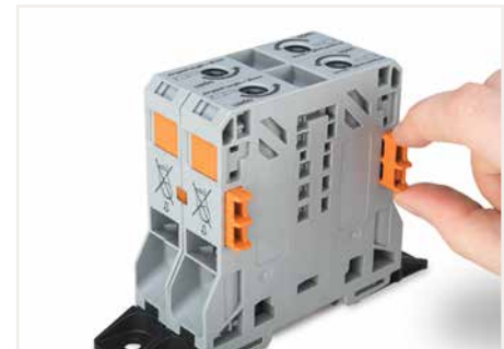
Optionally, insert block-to-block connector (285-448) into housing slot.
