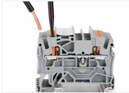
Terminating fine-stranded conductors via operating tool
