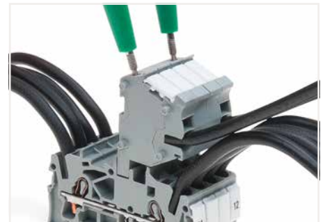
TOPJOB® S Connectors with a 2 mm Ø test socket for testing voltage via 2-pole voltage tester
