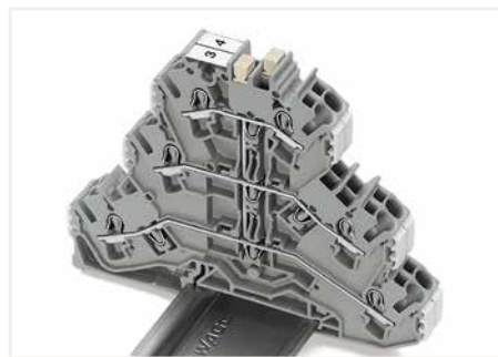
Commoning three levels via triple-deck vertical jumper (2002-493).
