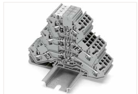
Triple-deck diode terminal blocks were specifically developed for custom diode circuits, such as lamp test and collective fault signal circuits. These terminal blocks provide high-density wiring in a width of just 5.2 mm. Push-in type jumper bars provide additional options for custom circuit design.
