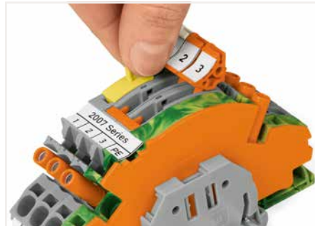
Lock-out prevents accidental operation of disconnect link.
