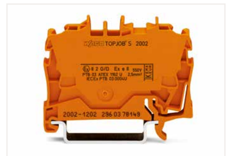
Example of marking (rear): The embossed details on the terminal blocks show the manufacturer's name, the series no., the type of protection Ex e II, the approval no., the approval data and the name of the testing authority.
