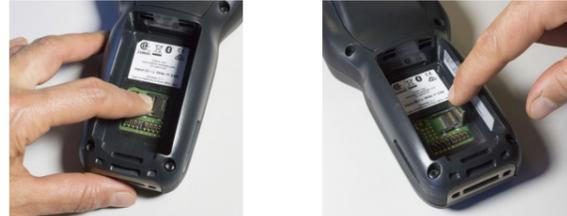
4. Insert the microSD card with the written part upward. Lock the card into place by pushing the cardholder down and then sliding it to the left:
