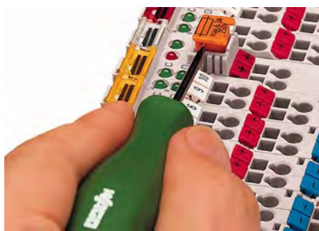
Figure 9: Removing the Fuse Carrier
