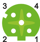
Figure 7: Network Connection, M12 Socket on Device
