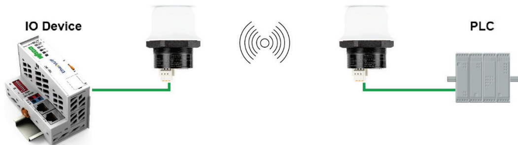
Figure 27: EtherNet/IP wireless network
