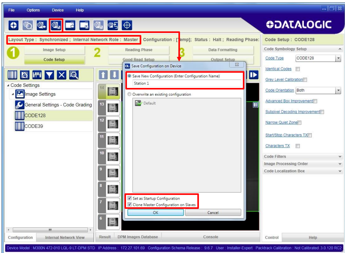
Figure 84 – Saving Synchronized Phase Mode Configuration to Master
