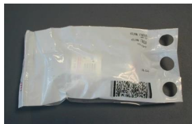
Figure 21 - Unidose Flow-Pack with PDF417 Code
