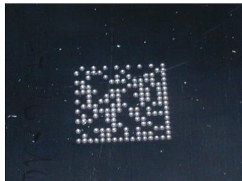
Figure 26 - Directly Marked Dot Matrix Code Characterized by Outstanding Separation Distance between Adjacent Code Elements
