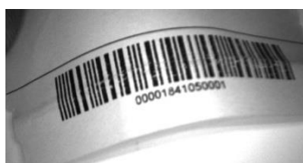
Figure 19 - Barcode Printed on Curved Surface Readable by Matrix 120 in spite of Image Optical Distortion
